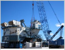
The displacement of large machines in surface mining requires a precisely planned approach. If a heavy, complex structure needs to be elevated, the lifting process must be controlled at all times. With the Dimetix laser distance sensors, the position of the lifted plant is measured permanently at different locations to ensure the structure always stays in an upright position.
